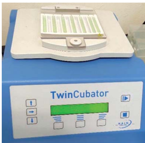
Fig. 4. Test strips incubated with amplified DNA and Hybridization Buffer on a TwinCubator shaker
