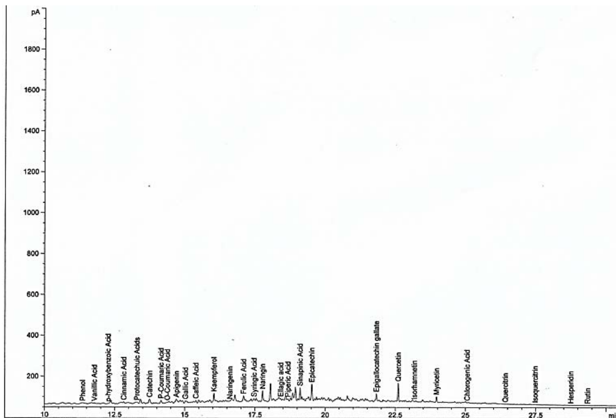
Fig. 2. HPLC-DAD Chromatogram of the phenolic contents of Pentaclethra macrophylla
